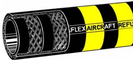
"Yellow Band" aircraft refuelling hoses, suitable for all aviation gasolines and jet fuels (JET A 1), deicing fluids or media and motor oils. Temperature range -30° up to +70° Celsius. Electrical resistance between 10<sup>3</sup> and 10<sup>6</sup> Ohm.
