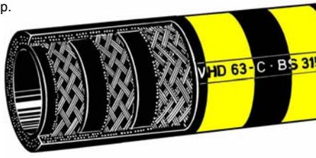
Special type "VHD" with three textile braids and thicker wall for lower bending radii and good suction rates. Burst pressure > 100 bar/1500 psi.
